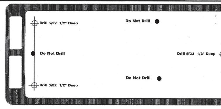
Door Jamb of INSWING - LEFT HAND HINGE - with Strike - Part Number 24-LK-30-P (wood frame) 24-LK-40-P (metal frame)
