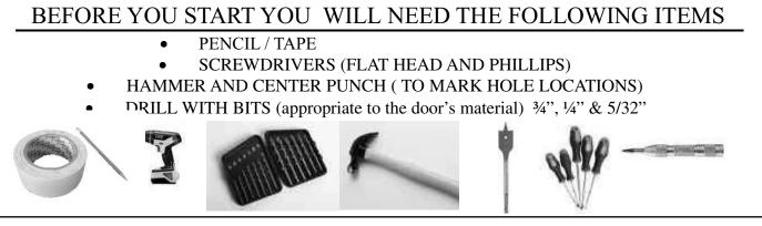
YOU MAY ALSO NEED A CHISEL TO MAKE AN AREA FOR MOUNTING THE STRIKE ON THE FRAME OF AN OUTSWING DOOR
